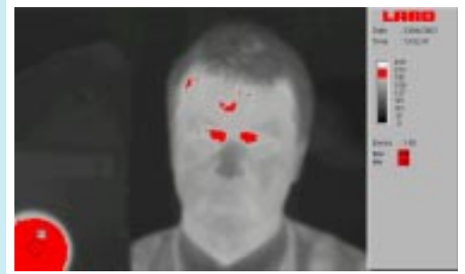
Isotherm function showing hot spots at the set point
