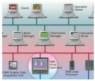
Visual Supervisor's control network provides peer-to-peer LIN communications with other control nodes such as Process Supervisors and additional Visual Supervisors. This communication is provided using ARCnet or Ethernet and is the method of connecting to Supervisory systems. Visual Supervisor can also be used to communicate with any third party device that supports Profibus DP and Modbus RTU protocol.
