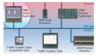
Visual Supervisor is designed to use Eurotherm's 2500 for its distributed I/O system. It can also communicate with any third party device that supports Profibus DP or Modbus RTU protocol.
