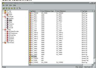
Eurotherm Project Studio 2000 contains the LINtools that is used to build both continuous and sequential control strategies and user screens. Eurotherm network explorer is also available to download files, and stop/start each individual Visual Supervisor node.
