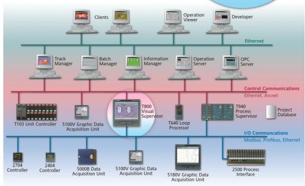
Visual Supervisor is an innovative multi-function control and display product. This product combines the well-established expertise, which Eurotherm has in control, data acquisition and process automation into a single product. It can be used either as a stand-alone system, or as a building block within a larger system. It can be connected to Eurotherm's proprietary ALIN local network, allowing both peer-to-peer and system communications.
