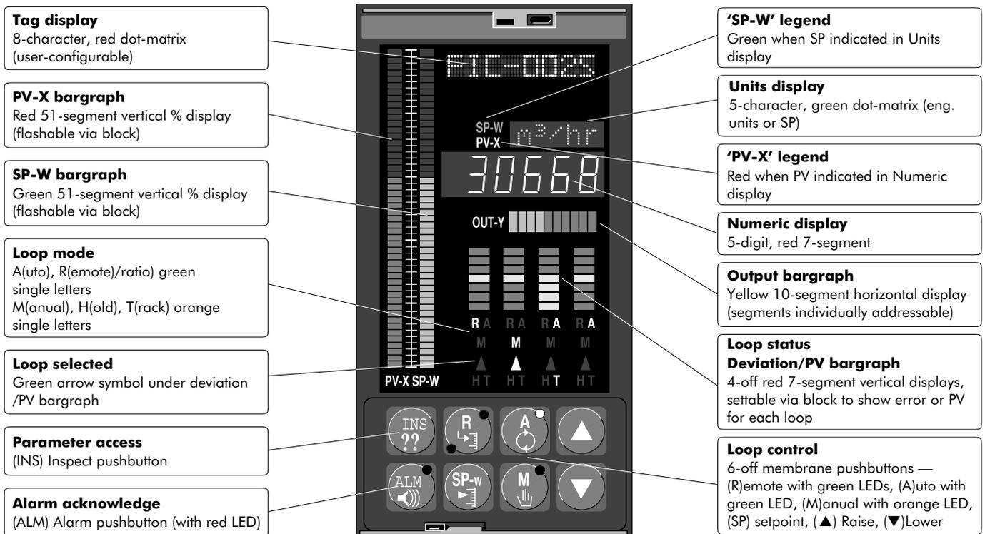
The main display shows the setpoint, process variable and output for the selected loop. These parameters are displayed on the bargraphs. The process variable is also displayed numerically on the five-digit numeric display. The standard control buttons operate on the selected loop.
